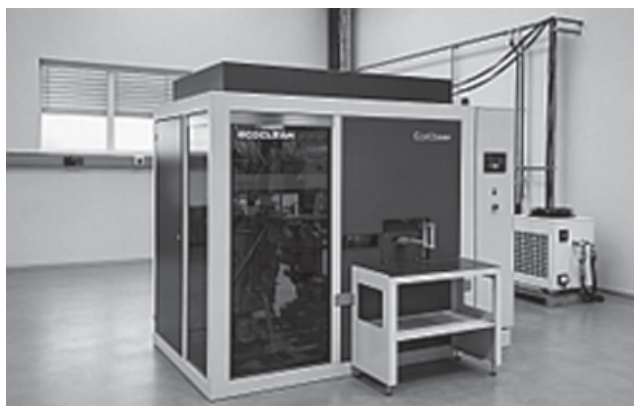
The EcoCbase was developed in S and M versions to provide a cost-effective way to begin using non-halogenated hydrocarbons and modified alcohols for powerful, economical, and reliable cleaning when cleaning volumes are low
