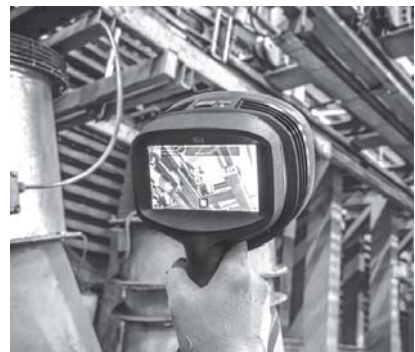
The FLIR Si2-LD detects two sources of potential compressed air leaks, distinguished from background noise
