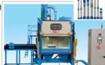
Spl. Blasting M/c for Cleaning of Submersible Pump Casing
