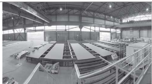
The preservation line with shot blast machine and automatic paint system can handle work pieces weighing up to 12 tons. The design was adapted to the existing building containing an overhead crane.
