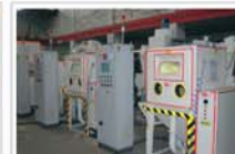
Spl. Shot Blasting M/c for Gear Cutters Tools before PVD Coating
