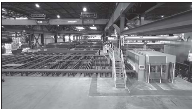
The preservation line with shot blast machine and automatic paint system can handle work pieces weighing up to 12 tons. The design was adapted to the existing building containing an overhead crane.
