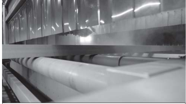
At the entrance to the automatic paint system special sensors measure the dimensions of the work pieces – down to the last mm.
